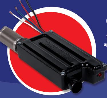
The Air Actuated® electric trailer brake controller provides smooth brake actuation. The electric brakes on the trailer operate off the air brake system of the tow vehicle. When the brake pedal is depressed, the application of the electric trailer brakes is proportional to the vehicle's brake pedal pressure.
